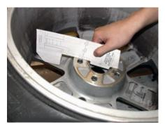
5. Lay the template inside the wheel as shown.
